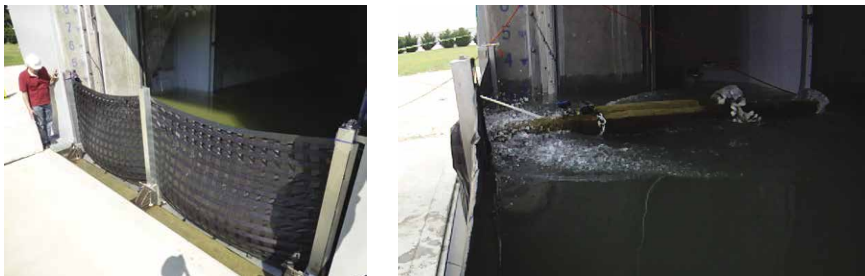
Figure D-14. Testing flex wall system.
