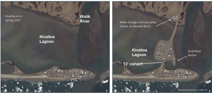
Figure 7-16. Original concept plan view of Kivalina Lagoon–crossing causeway and bridge design, Kivalina, AK; left panel shows before; right shows after and includes a new gravel pad island with a small boat harbor and an evacuation center and water storage at the end of the causeway. Source: Smith (2008).
