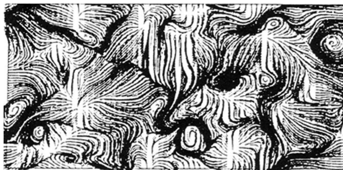
Fig. 12. DNS of instantaneous streamlines at free surface of open-channel flow (reprinted from Pan and Banerjee 1995, with the permission of AIP Publishing)
