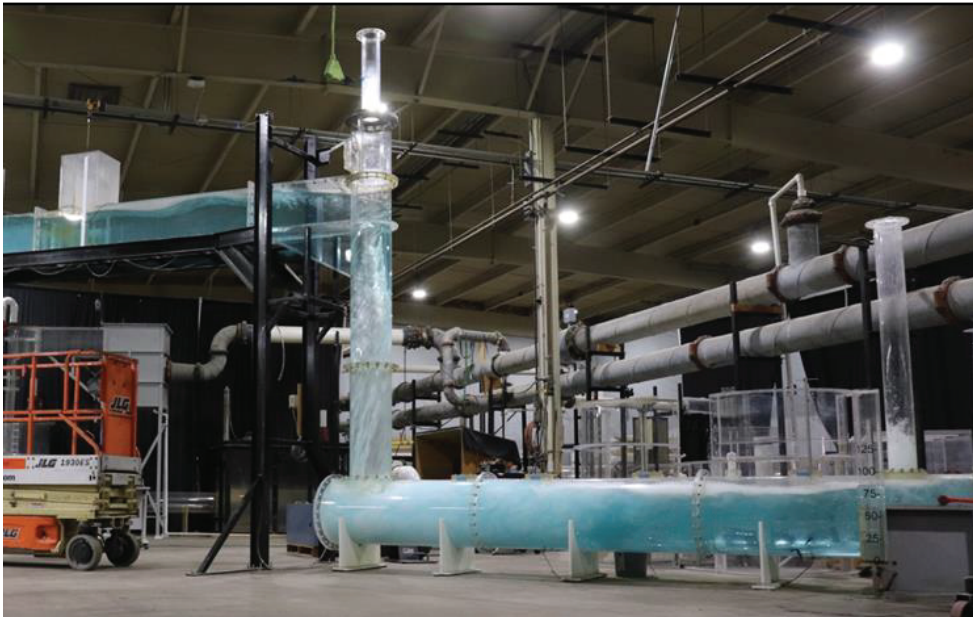
Figure 3.1 | View of the 16-length-scale physical model of the vortex intake and dropshaft and deaeration chamber used to aid design of the vortex intake and dropshaft for the Lower Middle River Des Peres, Combined Sewer Overflow, Storage Tunnel Project. This view shows the model in operation. (Scale = prototype/model).
