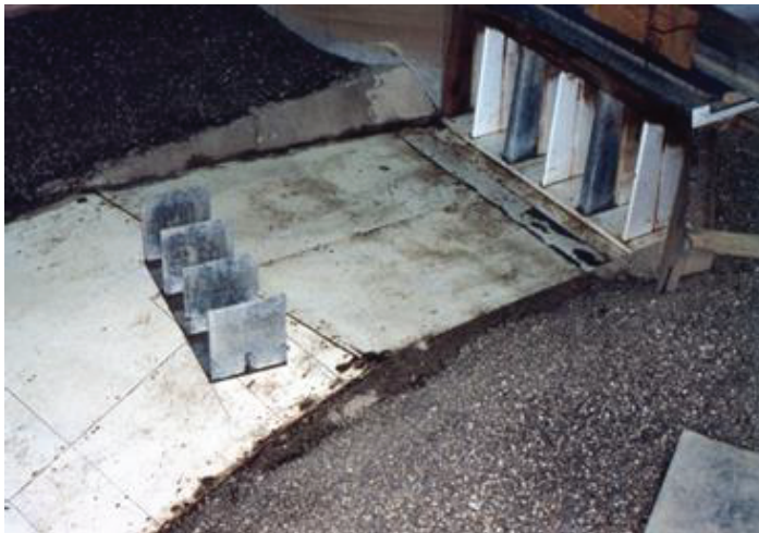
Figure 6.7 | A view showing a trial set of flow-guidance vanes used for flow straightening at the entrance of a prospective, run-of-river hydropower plant. (Ettema et al., 1996).
