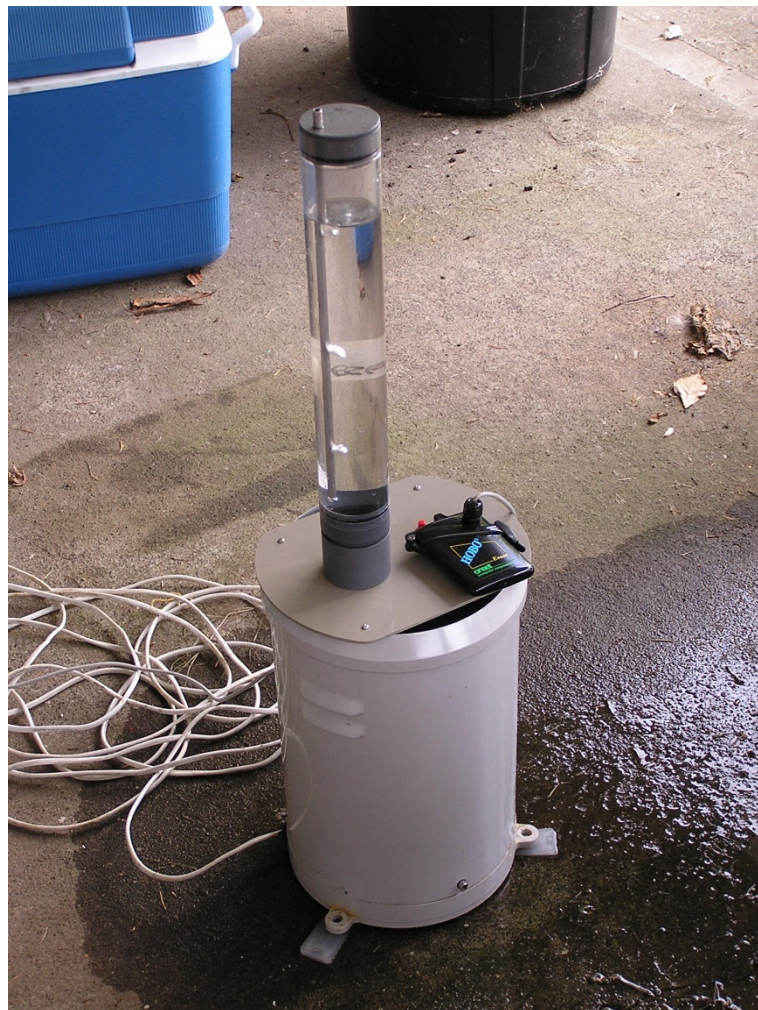
Figure 10. TB3 “tipping bucket” rain gauge calibration with a Hydrological Services TB320 Field Calibration device and a Hobo event recorder
