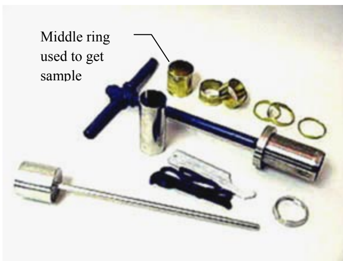
Figure 6. Soil corer used for taking soil bulk density samples - source ICT International
