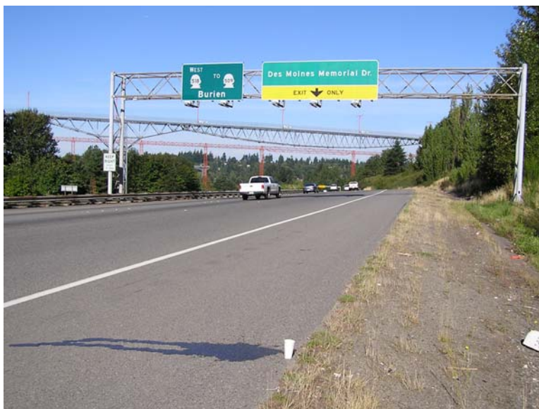
Figure 7. Water poured on the shoulder of SR 518 to determine the contributing area
