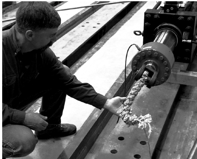
Figure 4. Failed test segment showing break at the end of splice (far end), spiral compaction of recoiled rope segment (original length about 10 feet between failure and pinned eye shown), and testing apparatus.
