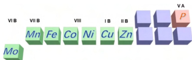
Fig. 5. Elements that are used to form TMPs for supercapacitors.
