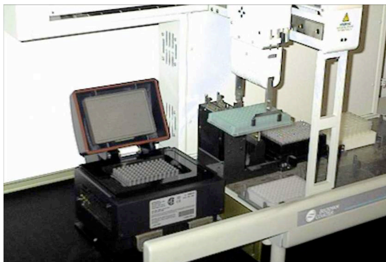
Figure 7: Use of gripper to pick up plate and re-locate it
