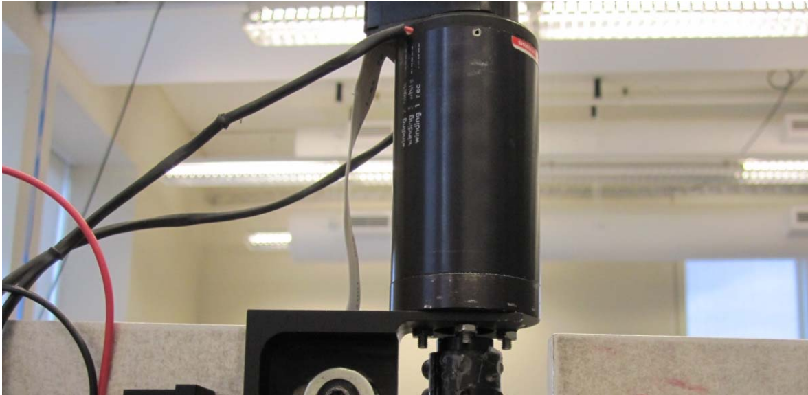
Figure 5. Actuator – Brushless DC Motor.
