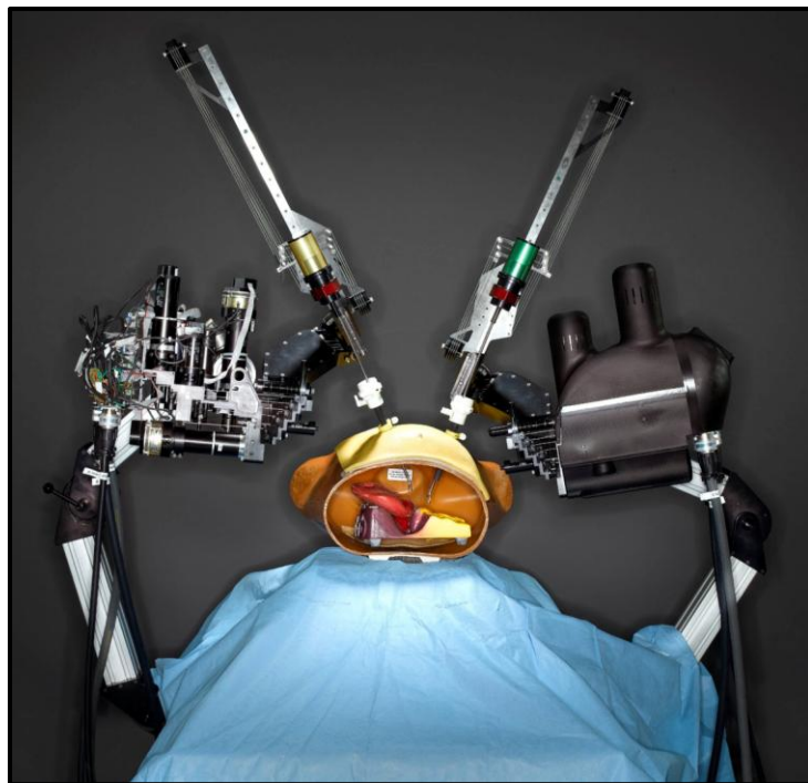
Figure 2. RAVEN remote surgical robot
