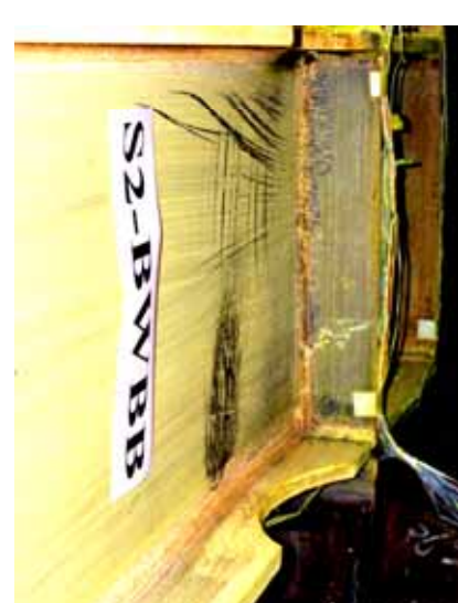
DS 5: Boundary Element Local Buckling
