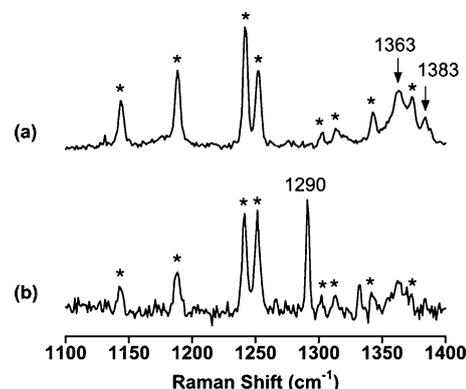
**Figure 3.** Resonance Raman spectra of **A** for samples prepared from a) <sup>16</sup>O<sub>2</sub> or b) <sup>18</sup>O<sub>2</sub> in THF at −80 °C (λ<sub>ex</sub> = 406.7 nm, 77 K). Solvent peaks are marked with an asterisk.
