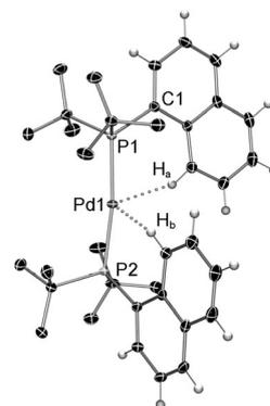
**Figure 1.** POV-Ray<sup>[15]</sup> rendition of the X-ray structure of **1** with thermal ellipsoids set at 50% probability and hydrogen atoms on the *t*Bu groups omitted for clarity. Selected bond lengths [Å] and angles [°] for **1**: P1–Pd1 2.2973(3), P2–Pd1 2.2917(3), P2–Pd1–P1 172.615(11), C1–P1–Pd1 118.16(4).
