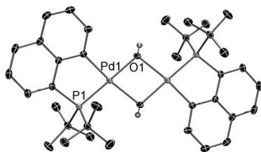
**Figure 2.** POV-Ray<sup>[15]</sup> rendition of the X-ray crystal structure of **2a** with thermal ellipsoids set at 50% probability. Hydrogen atoms (except on OH groups) and co-crystallized [D<sub>6</sub>]benzene omitted for clarity.
