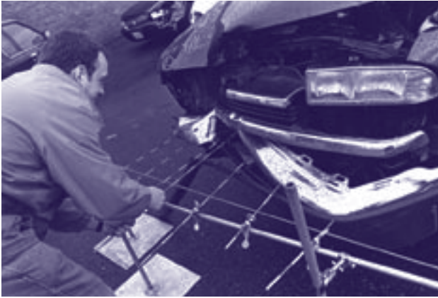
FIGURE 4. Seattle CIREN (Crash Injury Research and Engineering Network) site crash investigator examines crashed vehicle for clues as to causes of injuries to occupants.
