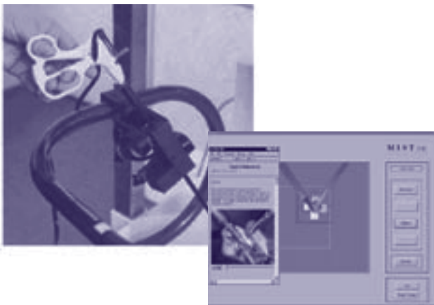
FIGURE 1: MIST-VR basic surgical skills simulator illustrating the image on the simulator screen, and the input handles for tracking motion
