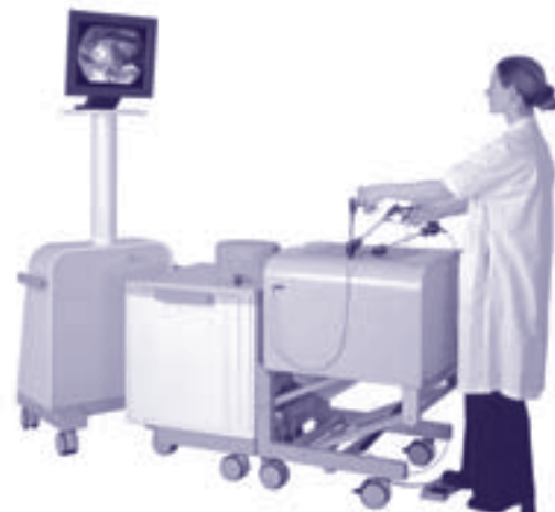
FIGURE 2: Xitact Laproscopic Cholecystectomy simulator illustrating the portable system and video image.
