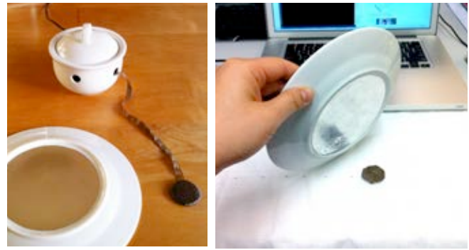
Figure 4: Sensing experiments: plate is coated with conductive material on the bottom and sits on a coin-sized soft conductive pad. The weight of the plate completes the connection. Additional ceramic housing for Sensing Plates (left).
