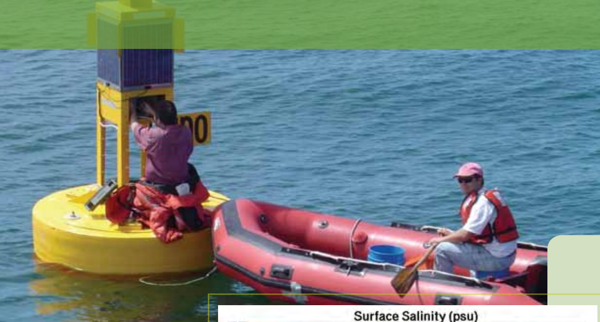
Above: OHSU field staff members Michael Wilkin and Jon Graves rewire an ocean observing buoy on a calm day in the Pacific Ocean west of Seaside, Oregon. Photo: Courtesy of CMOP
