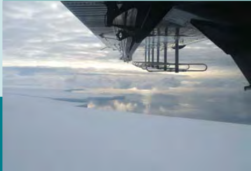
Below: Radar depth sounder antenna array mounted below the Twin-Otter wing during flight operations in Antarctica in 2010. Photo: Cameron Lewis
