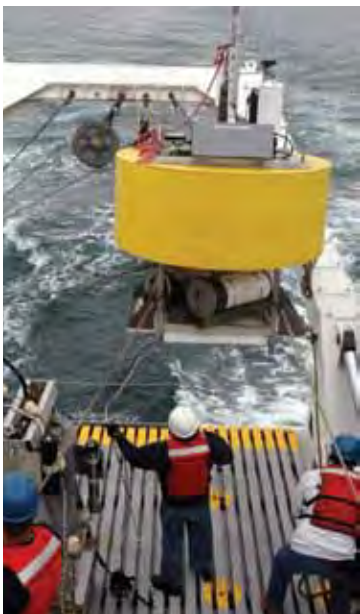
Deployment of the Environmental Sample Processor (ESP). Photo: Philip Sammet copyright 2010 MBARI.
