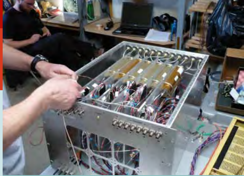
CReSIS Deputy Director Carl Leuschen performs in-the-field repairs to the depth sounder at Byrd Camp, Antarctica in 2010. Photo: Cameron Lewis
