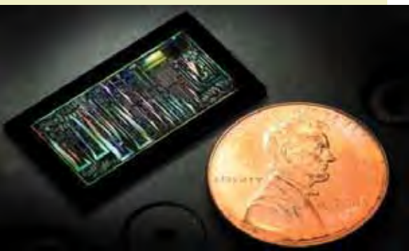
A photonic circuit next to a penny. Photo: University of Washington
