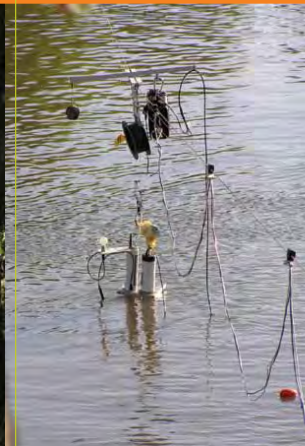
Water quality and flow sensors positioned at the surface of the river.
