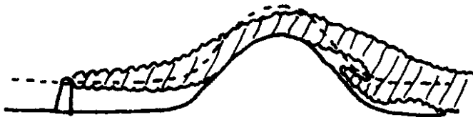
c) a more realistic possibility -includes possibility of an eddy in lee of hill -should include flow around the hill
