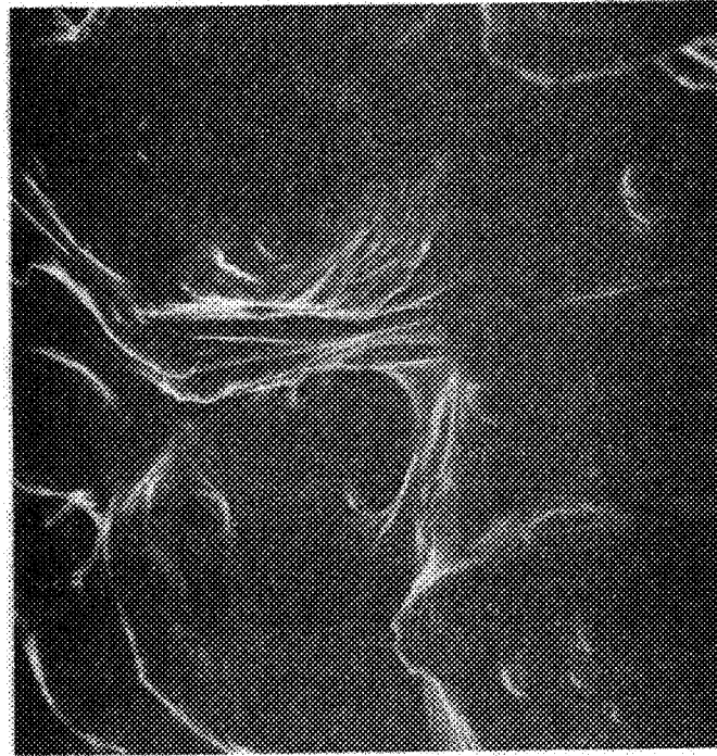
Figure C28. SEA 30/70 Mixture (AR-2000, crushed basalt, Marshall compaction) After Heat Soaking (585x)
