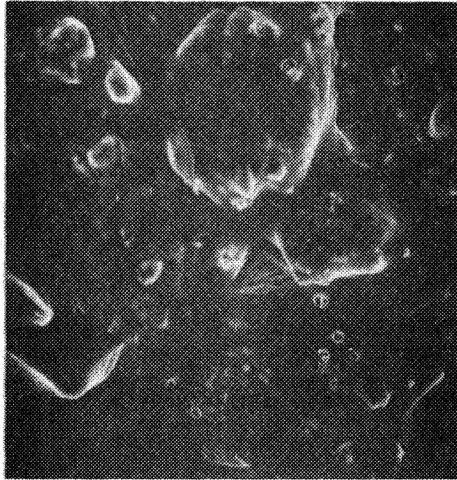
Figure C33. SEA 30/70 Mixture (AR-2000, crushed basalt, Marshall compaction) After Lottman Conditioning (510x)
