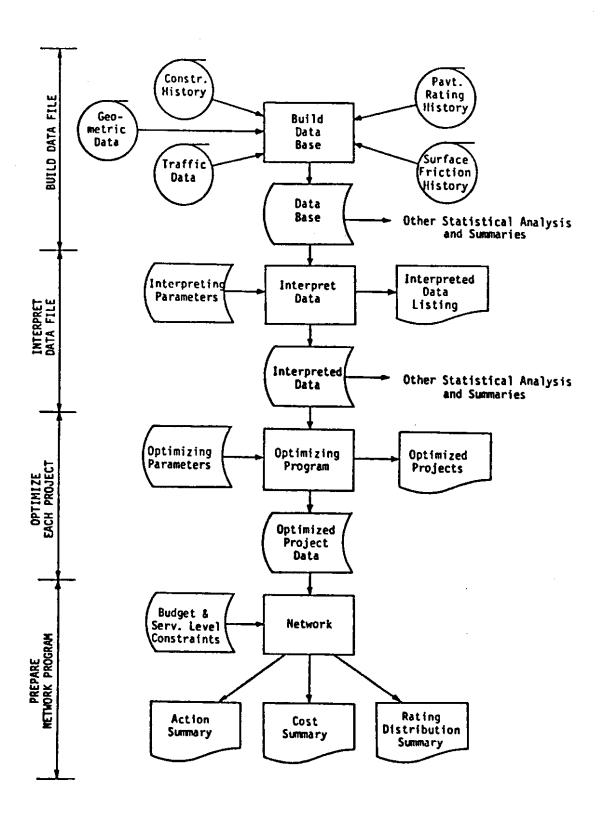
Figure 1. CONCEPTUAL FLOW CHART OF WSPMS OPERATIONS (Ref.1)
