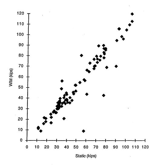
statistical difference in the percentage of error in a gross weight estimate was apparent between heavy trucks and lighter trucks at Pendleton and Snoqualmie, but that heavier vehicles were weighed more accurately (in percentage terms) at Nisqually and Martin Way.
