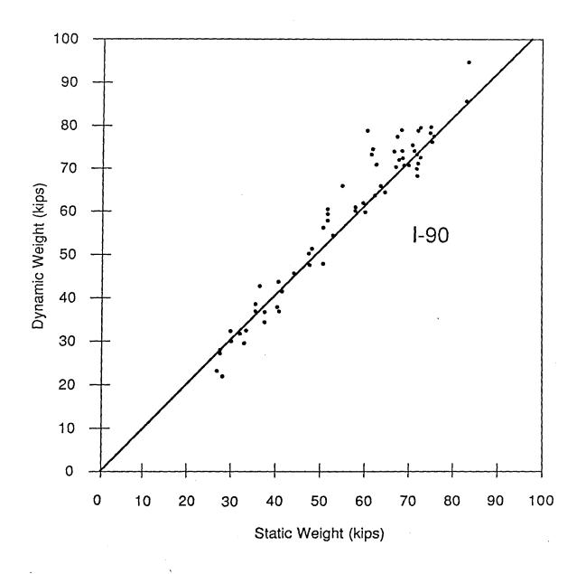
These results indicate that the estimates obtained with the WIM system were randomly oriented around the static estimate, but that the average errors were slightly larger than the repeatability tests indicated.
