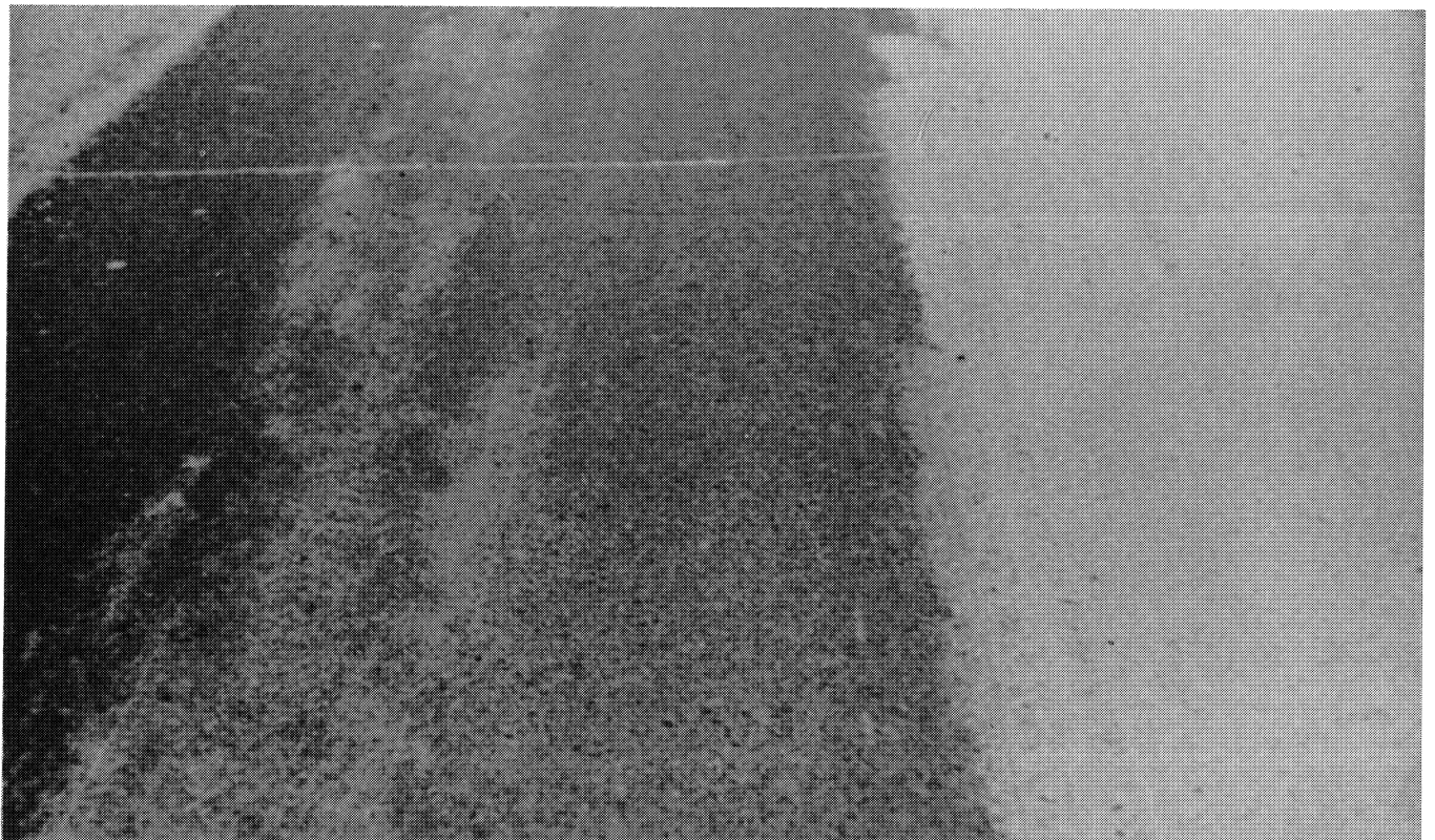
Figure (7) and (8) Interstate 90 forty minutes after CMA application at 29 degrees
