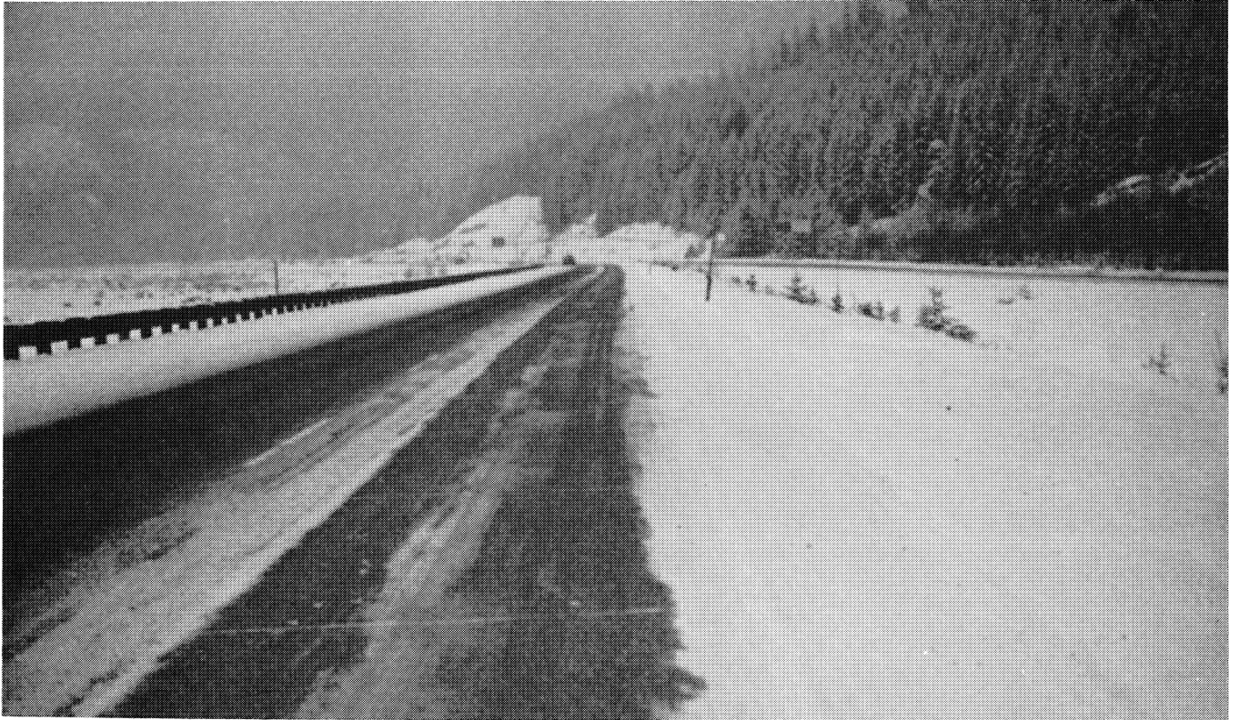
Figure (7) and (8) Interstate 90 forty minutes after CMA application at 29 degrees
