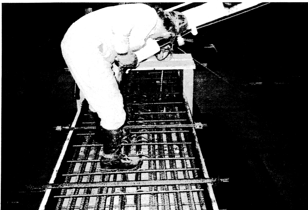
Figure 6.12 Laboratory Test - Placing Concrete in the Forms
