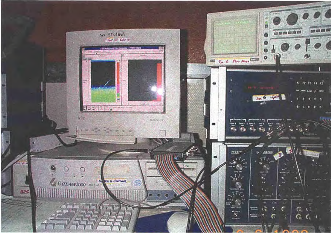
Figure 14. Real-time display of hydroacoustic "targets" detected by the single-beam transducers at the Port Townsend ferry terminal
