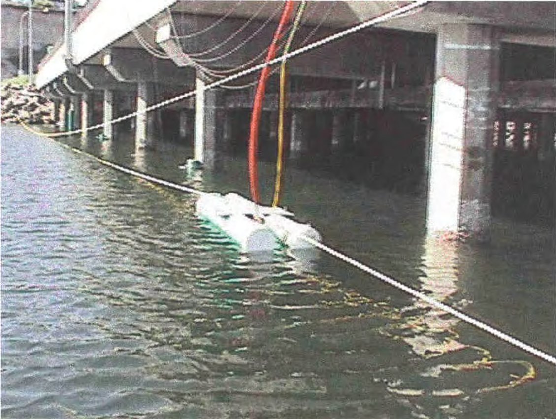
Figure 15. The underwater video system deployed at the Port Townsend ferry terminal from June 9 to 11, 1999
