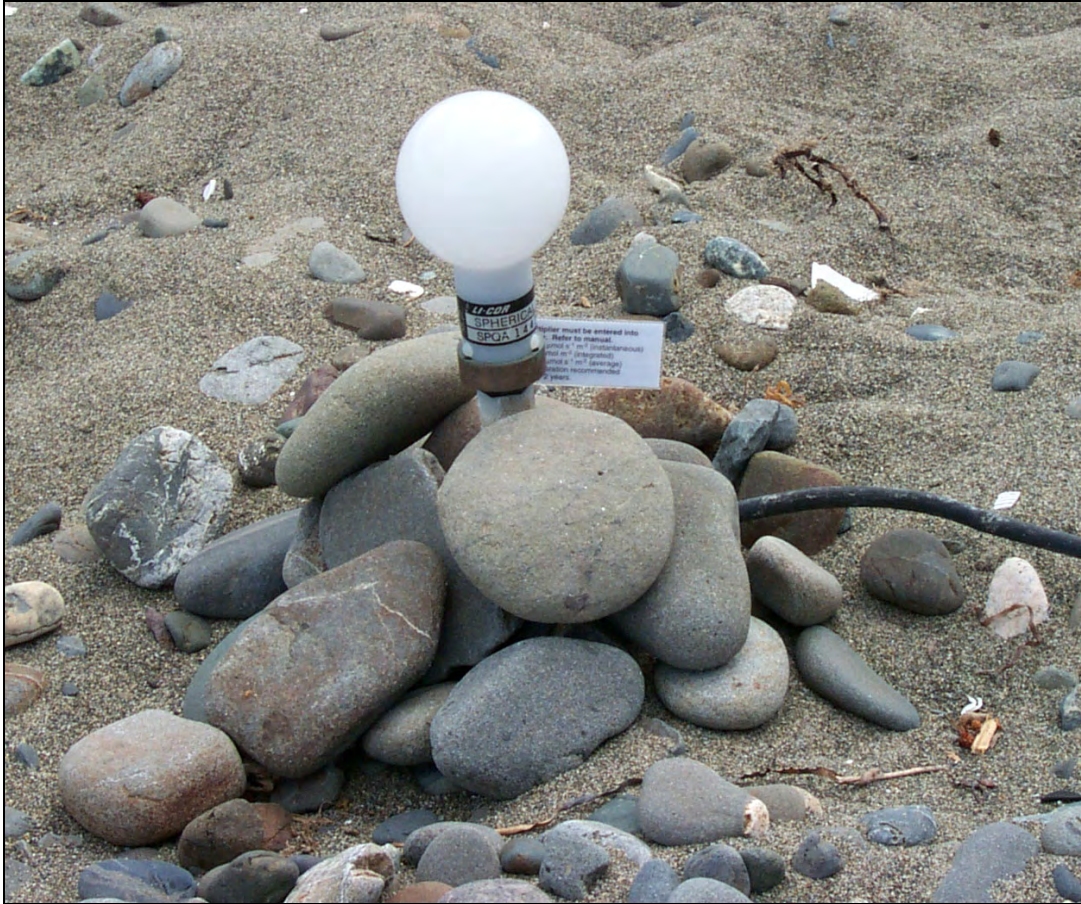
Figure 16. The LI-COR LI-193SA spherical quantum sensor that we used to measure photosynthetically-active radiation (PAR) at the edge and underneath the Port Townsend ferry terminal (Photo taken at Edmonds ferry terminal)
