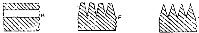
Figure 4 Thnadner barriers, Sawtooth (S) with 50% open, Flat-top (F) with 25% open, & H design.
