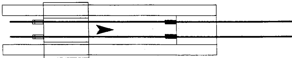
(c) Lock front chucks to hold tension and retract ram.
