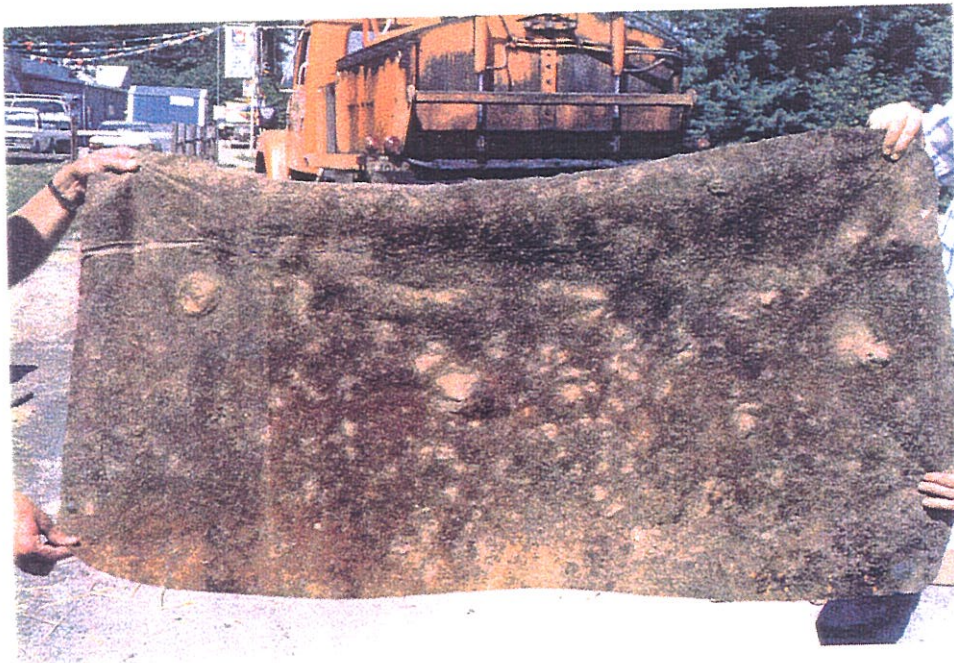
Figure 5.83 - Bottom surface of the exhumed geotextile.
