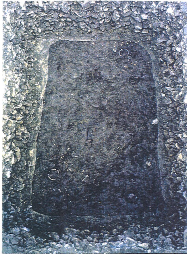
Figure 5.21 - Exposed subgrade with driven Shelby tube samples.
