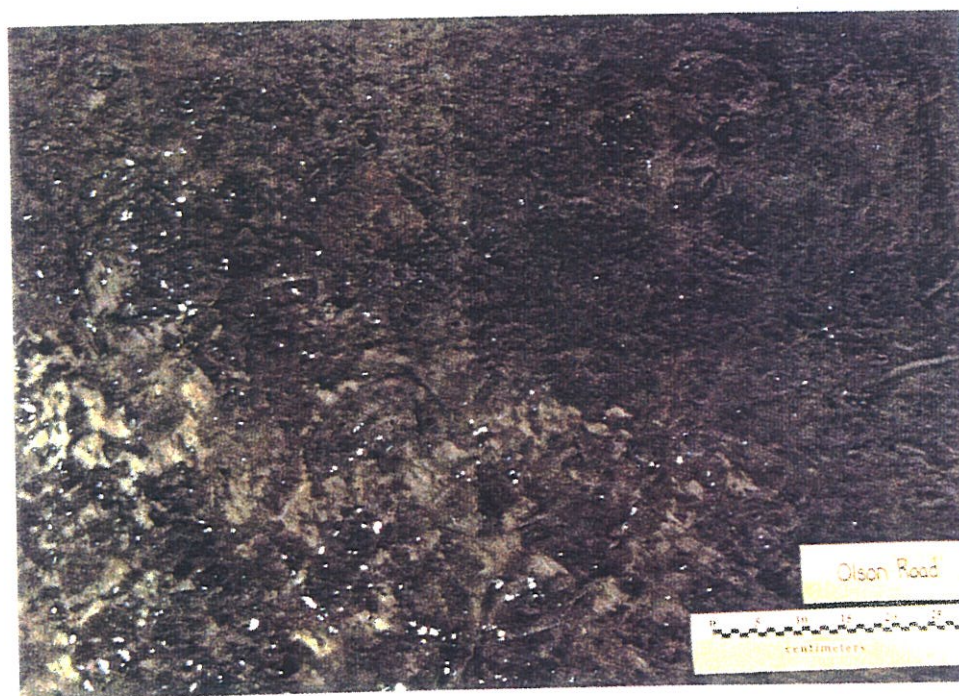
Figure 5.96 - Middle area of the bottom surface of the geotextile showing the degree of damage. The top of the photo is the north side, right is west. Illuminated from behind.
