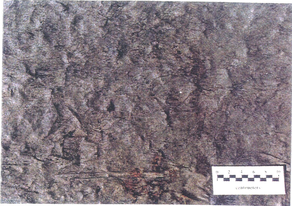
Figure 5.22 - Laboratory photograph of the bottom surface of the geotextile with a small iron stained area.
