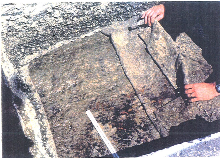
Figure 5.28 - Geotextile pulled back to expose the subgrade surface.
