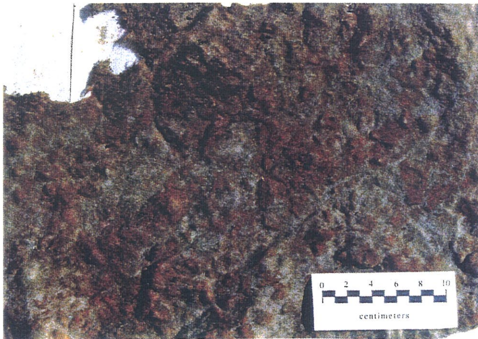
Figure 5.15 - Photograph of iron staining and condition of a relatively undamaged area on the bottom surface of the geotextile, testpit 1.
