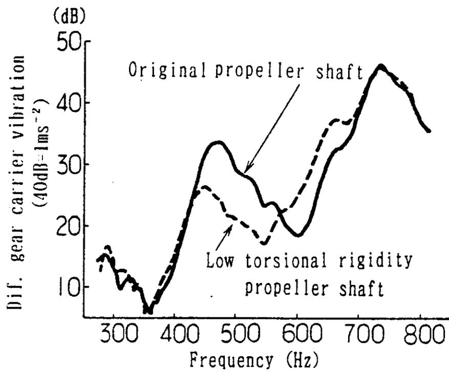
Figure 7. Effect of substituting a low torsional rigidity propeller shaft on gear vibration; from Reference [Hirasaka, 1991]
