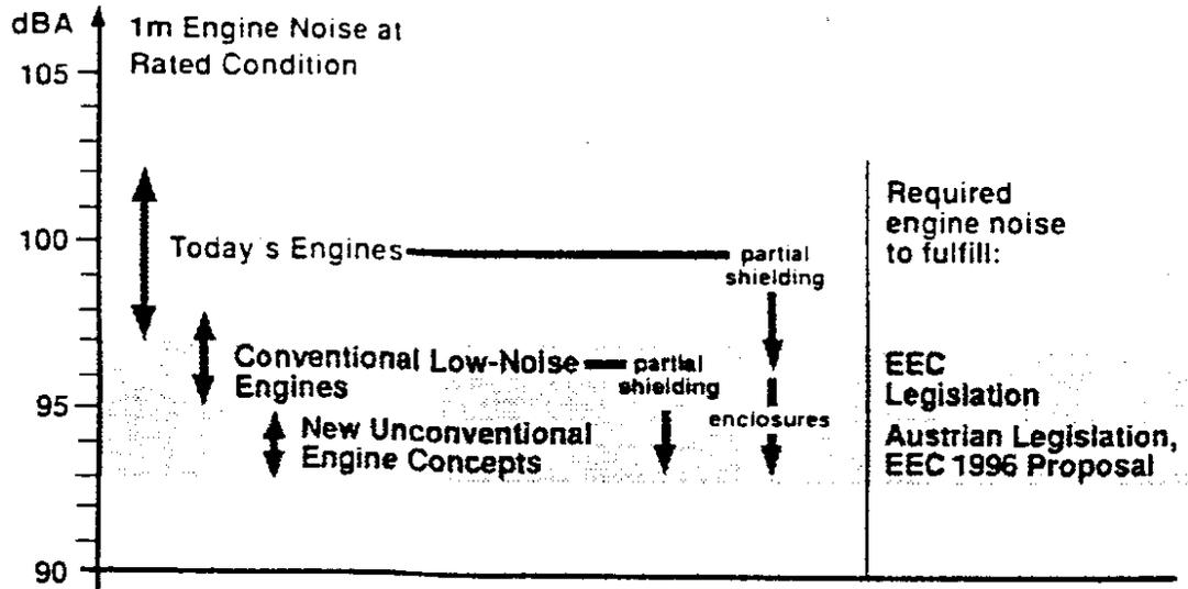
Figure 3. Reduction in engine noise levels to meet requirements of legislation; from Reference [Brandl, 1991]
