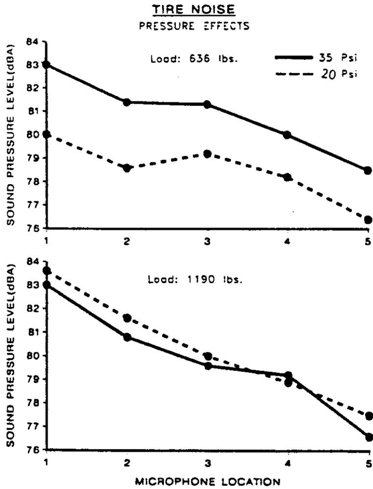
Figure 8. Effect of pressure on automobile tire noise; from Reference [Muthukrishnan, 1990]
