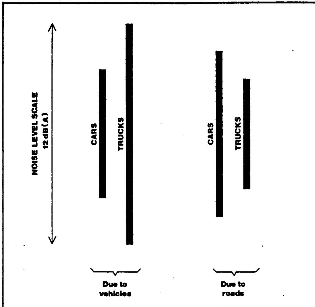
Spread in traffic noise on different road surfaces and from individual vehicles, according to measurements at VTI 1982-88 in free-flowing traffic at about 70 km/h. Only dry, bituminous road surfaces are included. The bars indicate approx. the 5 to 95 percentiles, i.e. there are generally 5 % more extreme values at either end.
