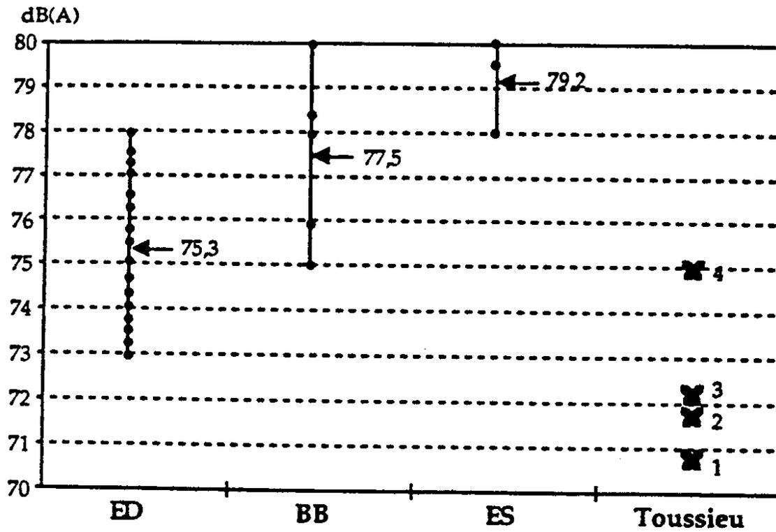
Reduction of car pass-by noise levels at 90 km/h
