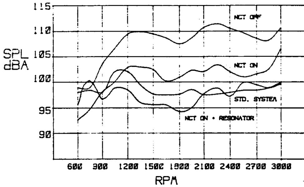
Figure 5. Exhaust noise levels for alternative exhaust systems; from Reference [Eghtesadi and Gardner, 1989]
