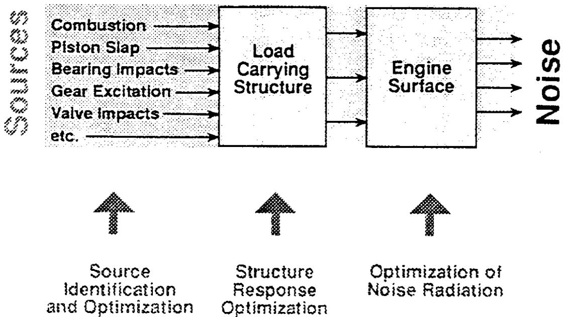
Figure 1. The noise generating process for engines; from Reference [Brandl, 1991]
