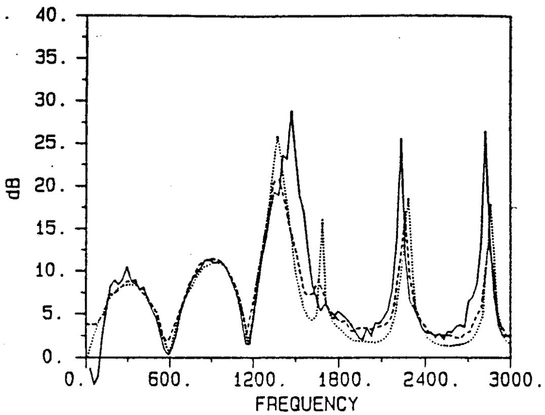
Figure 4. Frequency-dependent noise peaks for exhaust noise; from Reference [Morel, 1991]
