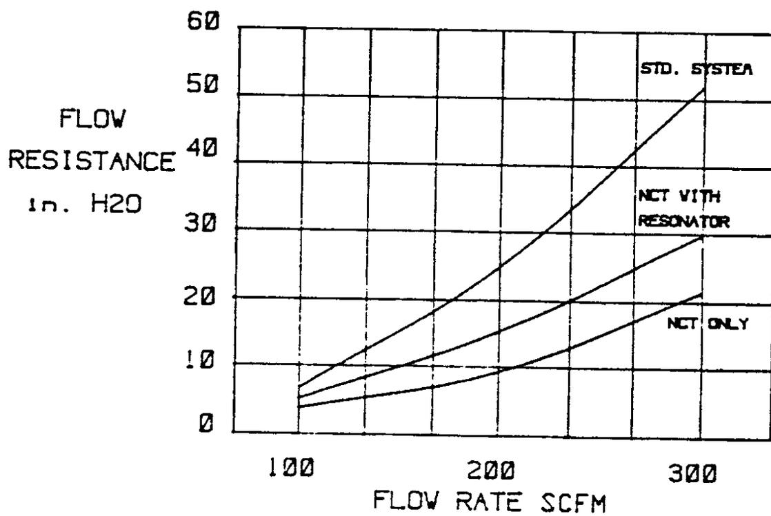
Figure 6. Exhaust back pressure for alternative exhaust systems; from Reference [Eghtesadi and Gardner, 1989]
