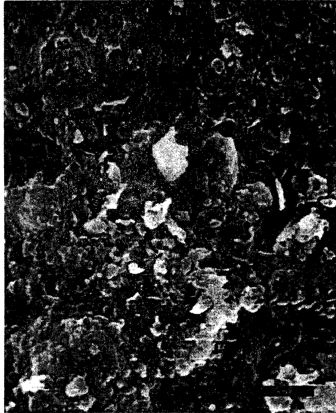
FIGURE A.2 SEM Micrograph of Everett Sand, 3 000 X. This photo of the sand surface shows evidence of plate-shaped particles attached to the surface of the larger sand grains. During batch sorption experiments, these particles appeared to be released, evidenced by a cloudy appearance in the liquid phase following agitation of the sample. A particle size distribution analysis of the particles showed that they had a mean diameter of about 1.5 mm, the approximate size of many of the attached particles shown in this photo. Although the release of the particles did not appear to introduce significant error during the batch sorption studies, their release in the subsurface may contribute to enhanced contaminant migration if they bind contaminants. It is unknown whether or not their release played a role in the column transport experiments performed in this study. However, no evidence of particle release from the column was observed by the naked eye.
