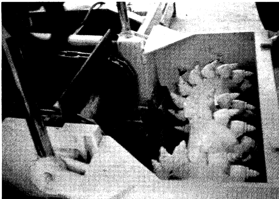
Picture 8. Milling head of "Unit B". Removes the material from the center portion of the lane that was not removed by "Unit A" (photo courtesy of Pacific Pavement Recycling, Inc.).
