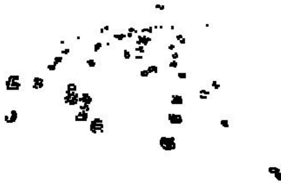
After dilation by a 3x3 structural element
