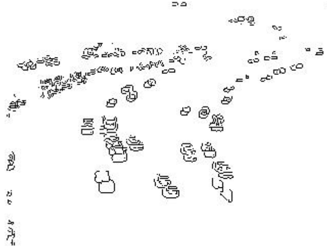
Figure 2.4 Sobel edges in the difference image between the first two frames
