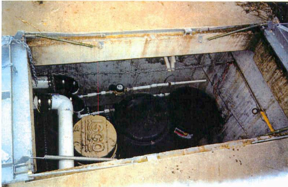
Figure 4. Photograph of sampling vault A with the ISCO sampler and plastic composite containers.
