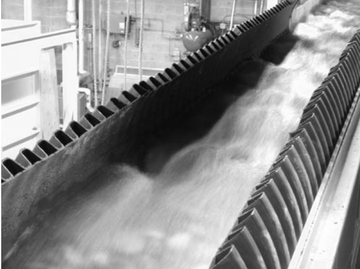
Figure A5. Time exposure of flow in the culvert, showing a typical step pattern formed in the bed.
