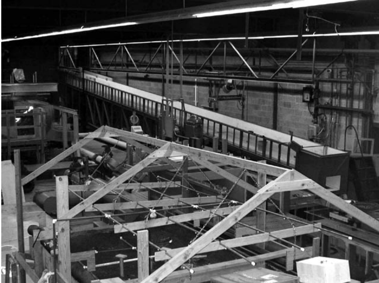
Figure A2. Top perspective of tilting flume (running diagonally across top of picture. Flume slope is 0.07 ft/ft.
