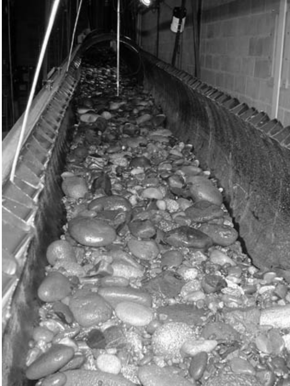
Figure A4. Gravel bed inside culvert, looking upstream. The Swoffer current meter is mounted on a rod in the center of the culvert. The D_{84} = 4'' gravel size distribution is shown here.
