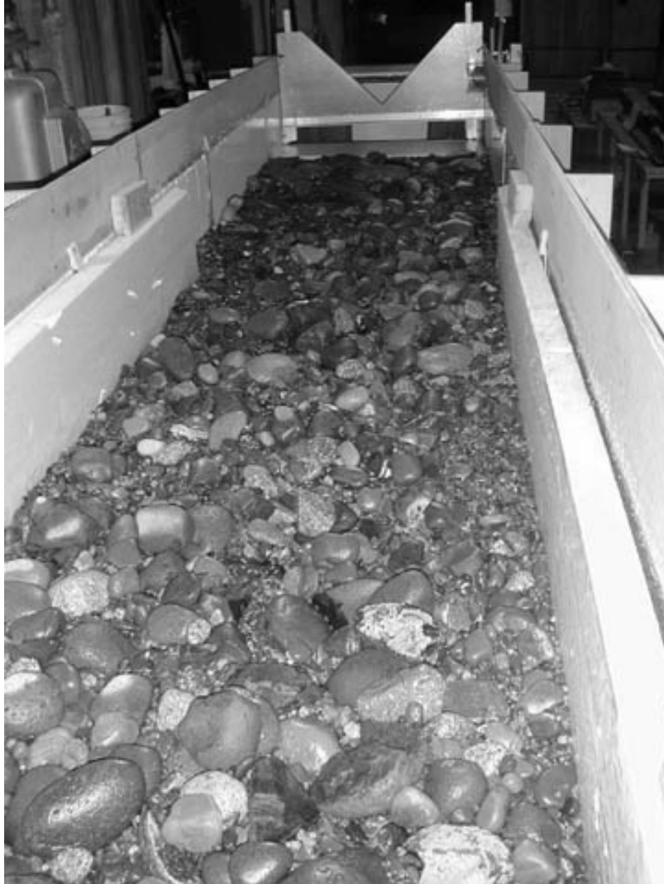
Figure A3. Gravel bed ( D_{84} = 4'' ) in place, looking downstream from culvert outlet. The V-notch weir used a water level control is visible at the tailgate of the flume, immediately preceding the sediment catchment system.
