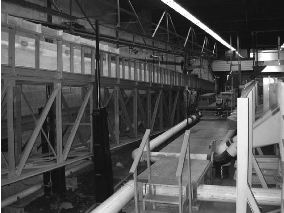
Figure A1. Side view of tilting flume, looking downstream (the flume is the structure at the left side of the image). The slope in the photo is approximately 0.07 ft/ft.
