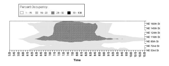
Figure 7: Occupancy Contour Map of Fuzzy Metering on I-405
