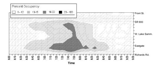
Figure 2: Occupancy Contour of Local Metering on I-90
