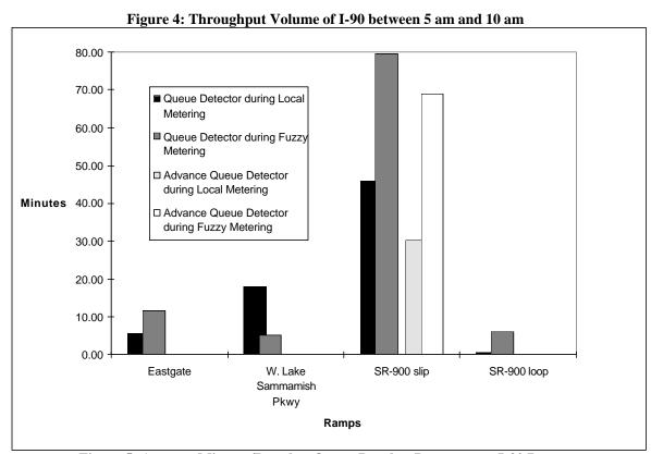
Figure 5: Average Minutes/Day that Queue Reaches Detectors on I-90 Ramps
