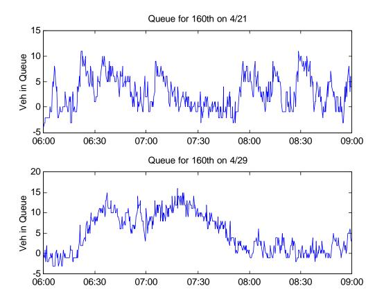
Figure 12: Vehicles in Queue at 160th for Bottleneck and Fuzzy Metering
