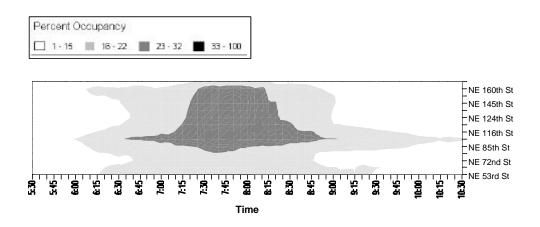
Figure 6: Occupancy Contour Map of Bottleneck Metering on I-405
