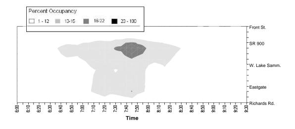
Figure 3. Occupancy Contour of Fuzzy Logic Metering on I-90
