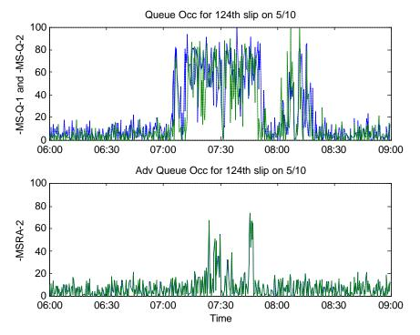
Figure 11: Queue and Advance Queue Occupancies during Fuzzy Metering at 124th
