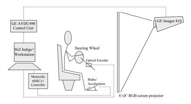
Figure 9.4: Driving simulator setup.
