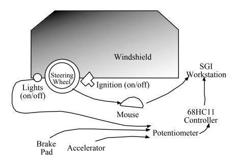
Figure 9.3: Components of the car used for the simulator.
