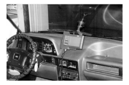
Figure 9.2: View of Trafficmaster mounted in car.
