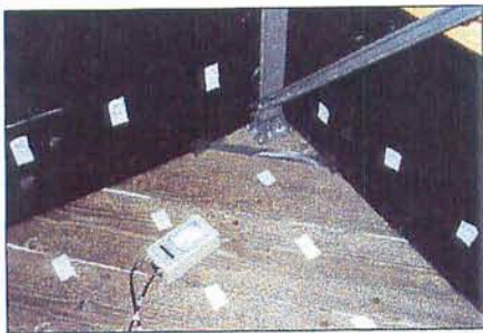
Figure 6. LI-COR data logger and diffusion sampling stations (white marks on the floor) inside the lightproof structure.
