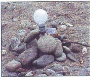
Figure 5. Spherical quantum PAR sensor by LI-COR
