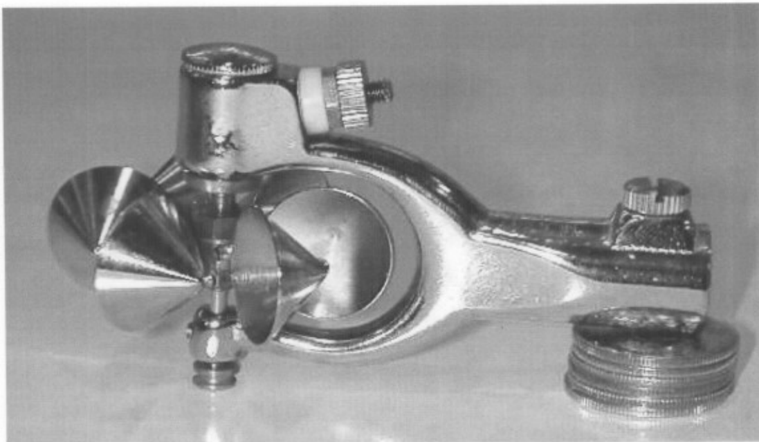
Figure A.5. Velocity Measuring Instrument: Pygmy meter (Note: quarter-size coin shown for scale)
