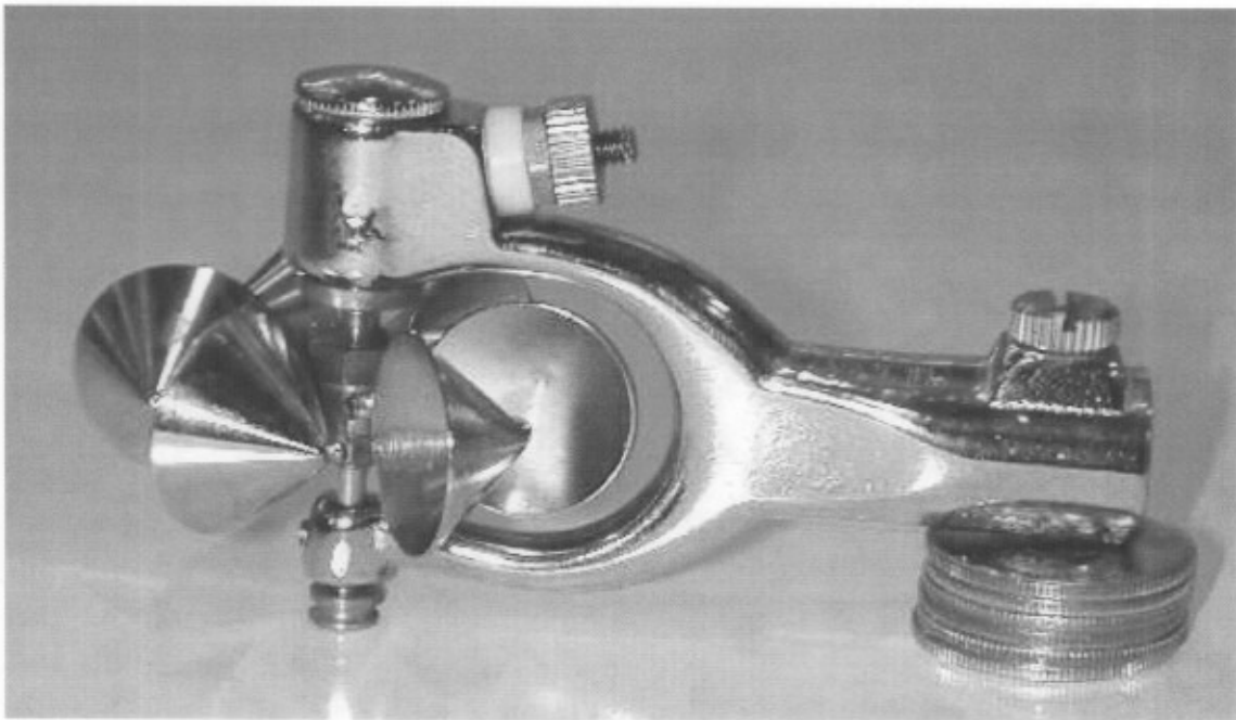
Figure 5. Velocity Measuring Instrument: Pygmy meter (Note: quarter-size coin shown for scale)
