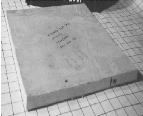
a) Category A - No Visible Damage
