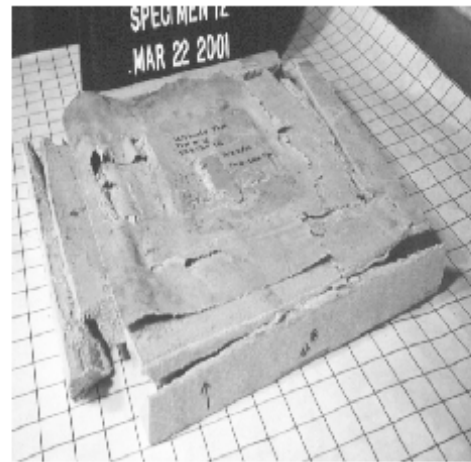
d) Category D - Diagonal Fracture
