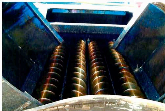
Photo 19. Auger system within the Novapaver.
