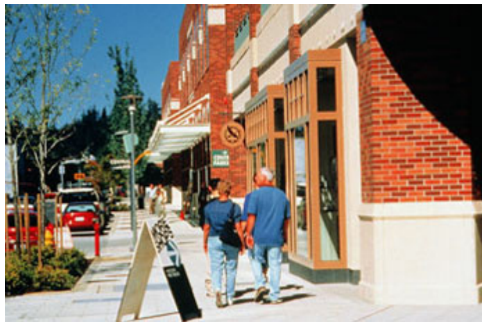
Figure V.11: Redmond, Wash. Awnings and overhangs are complementary to building design and provide pedestrian weather protection.
