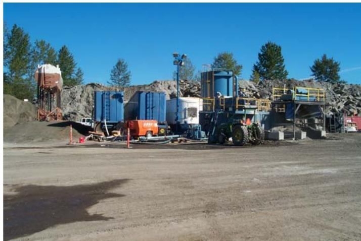
Photo 41. Processing plant for treating diamond grinding slurry.
