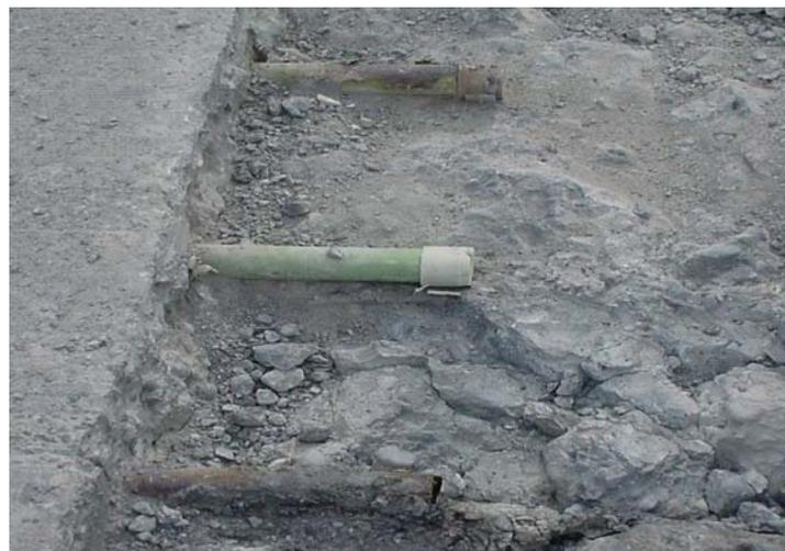
Photo 25. Epoxy coated dowel bars that had chips and nicks prior to placement. The corrosion, which resulted two years after placement, could have resulted from improper handling.
