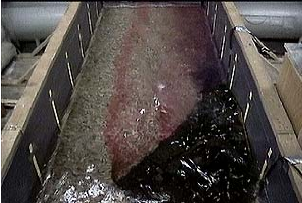
Figure 6. Flow in the vicinity of the rock barb biases the average velocities and makes instantaneous velocity measurements uncertain; and measurements contain correlations less than 70%, and are deemed poor, due to inadequate signal strength and excessive air bubbles (Nielsen et al. 1997).
