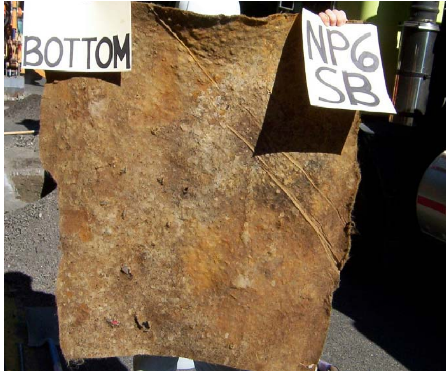
Figure 3.21. Bottom of NP6-SB geotextile after removal.
