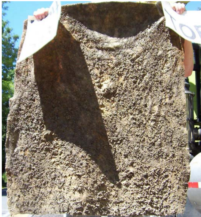
Figure 3.30. Top of NP4-SB geotextile after removal.
