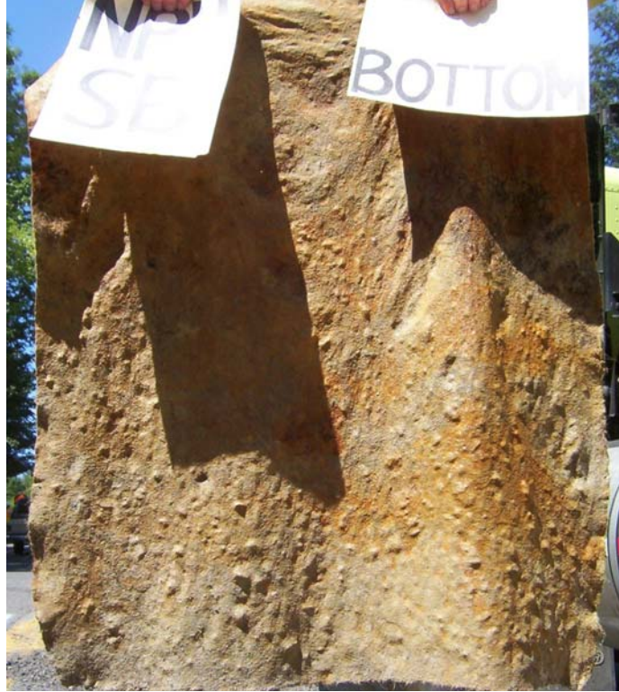
Figure 3.29. Bottom of NP4-SB geotextile after removal.
