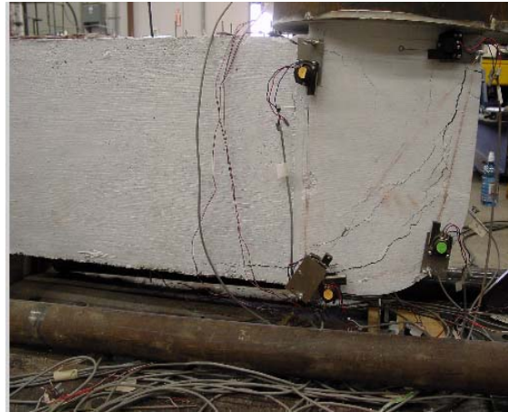
Figure 4-10: Crack Pattern in WSU Short and Long Outrigger, In-Plane Loading (Courtesy of Washington State University)
