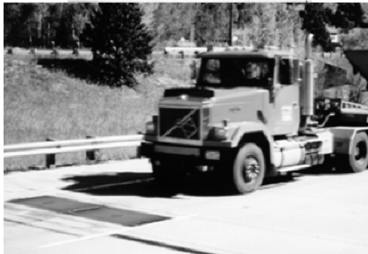
Figure 2-13. Single load cell (from International Road Dynamics Inc., www.irdinc.com )
