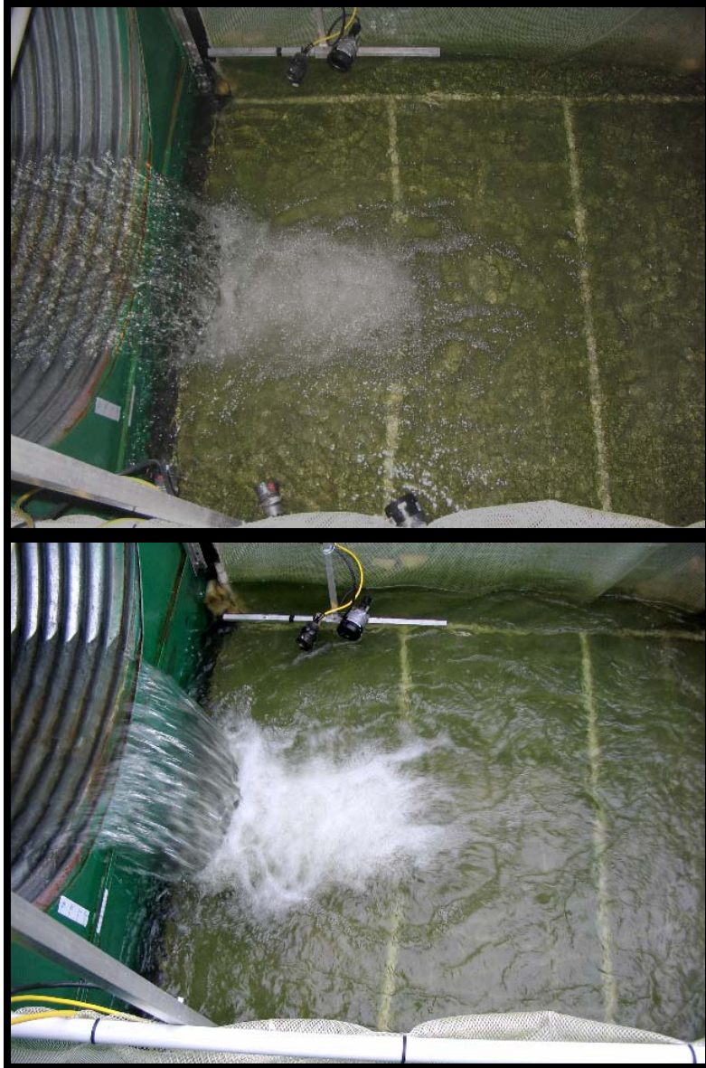
Figure 4. Culvert entrance with a 26-cm outfall drop (plunging flow, top) and 32-cm outfall drop (plunging flow, bottom)
