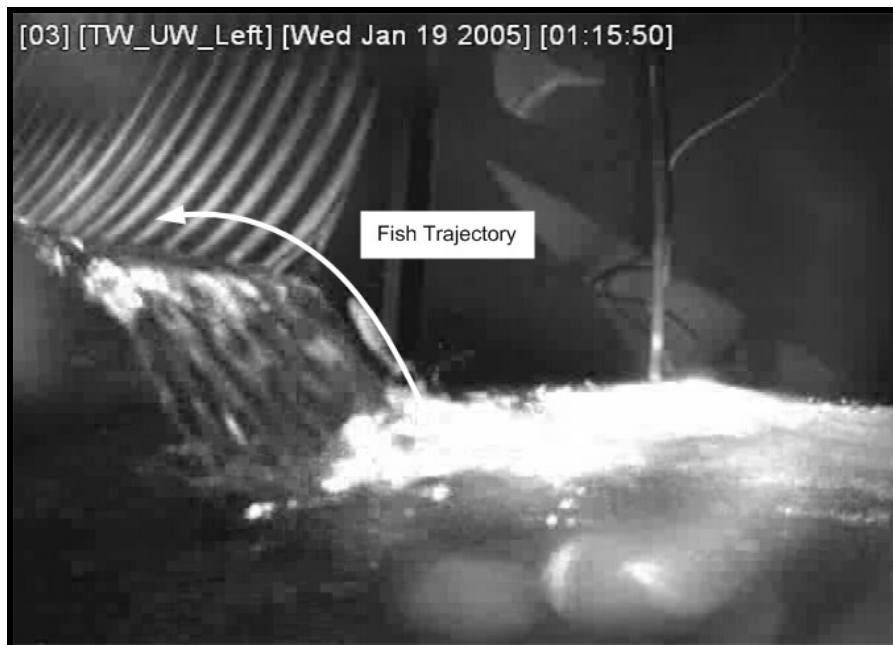
Figure 11. Example of a typical low-leap trajectory for a juvenile coho salmon leaping into the culvert set at a 20-cm outfall drop.
