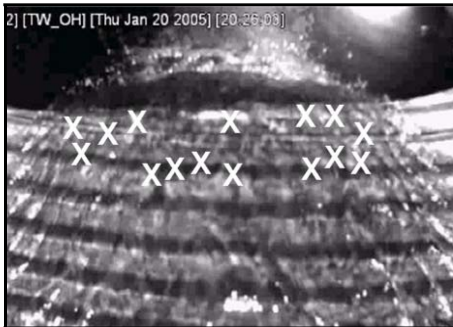
Figure 13. Overhead view of culvert entrance indicating where a sub-sample of fish landed inside the culvert after successful leaps (examples are from 12-cm and 20-cm outfall droptests). The wetted width of the culvert as shown is 76 cm.
