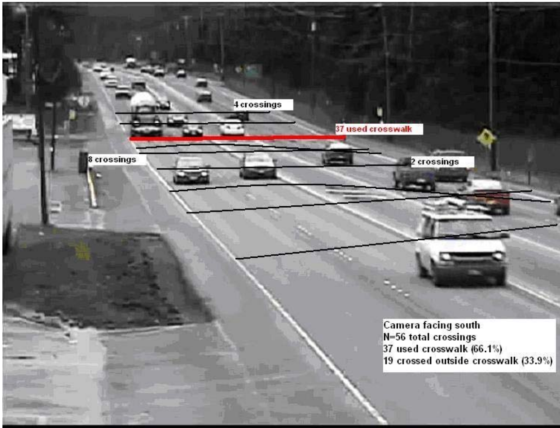
Figure 8. Pedestrian crossing paths to the south of S. 180 th Street
