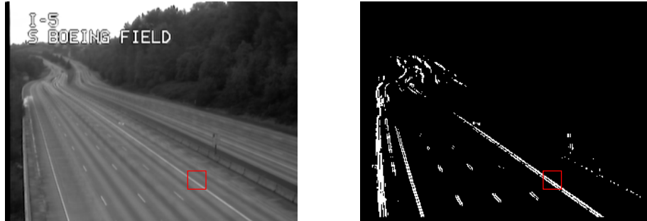
Figure 3.1: Background image on the left, thresholded edge image on the right.
