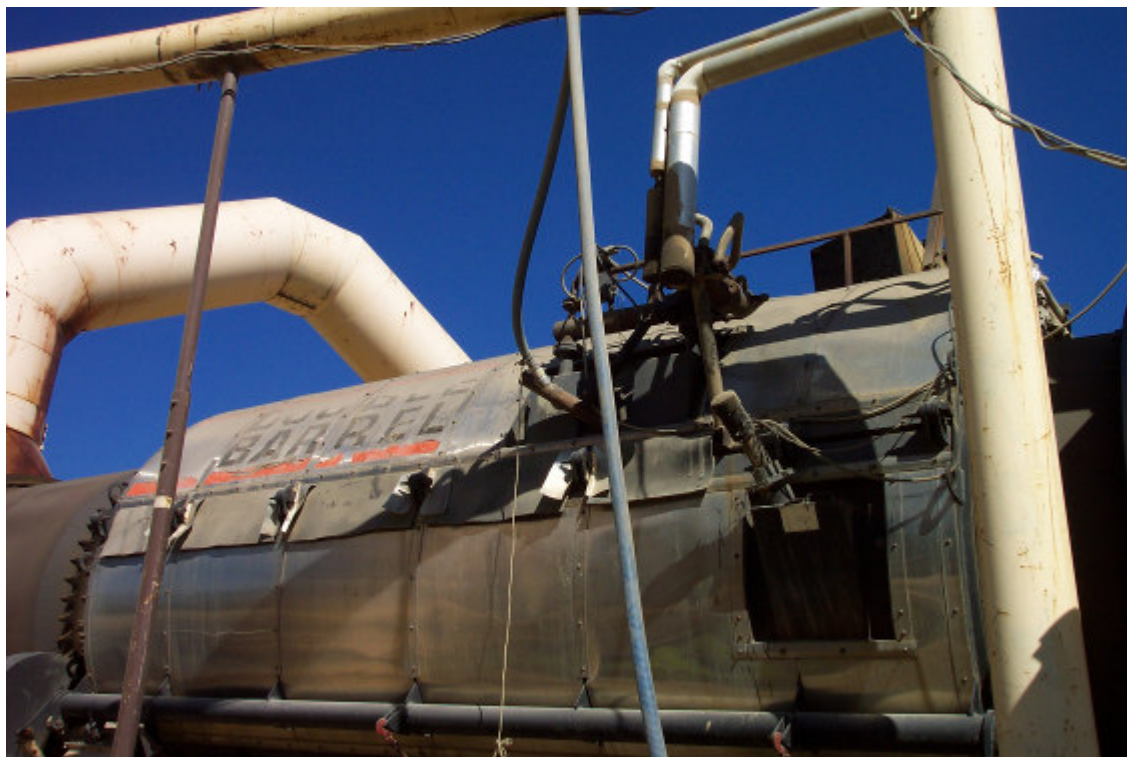
Figure 3.4: Plant retrofitted for Sasobit wax addition. [24]
