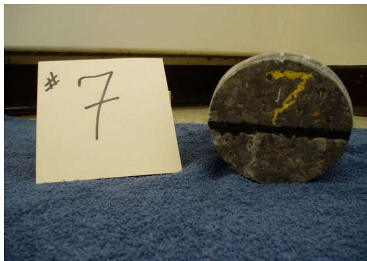
Figure 14. End view showing joint and crack. Aug. 04.
