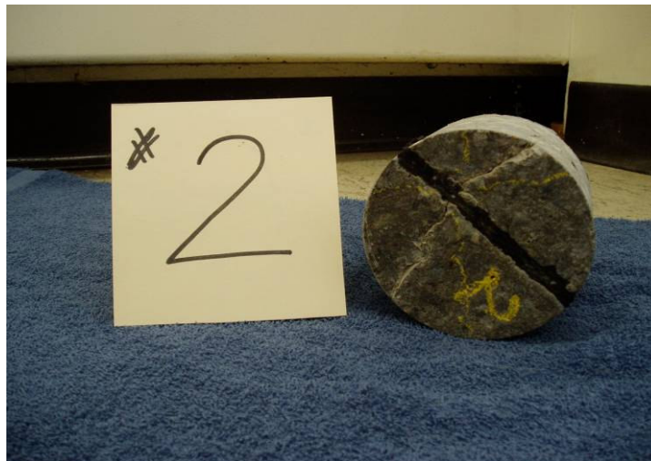
Figure 4. End view showing joint and crack. August 2004
