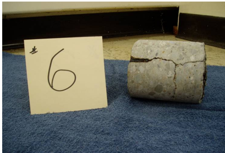
Figure 11. Side view showing panel joint and cracks. 8/04
