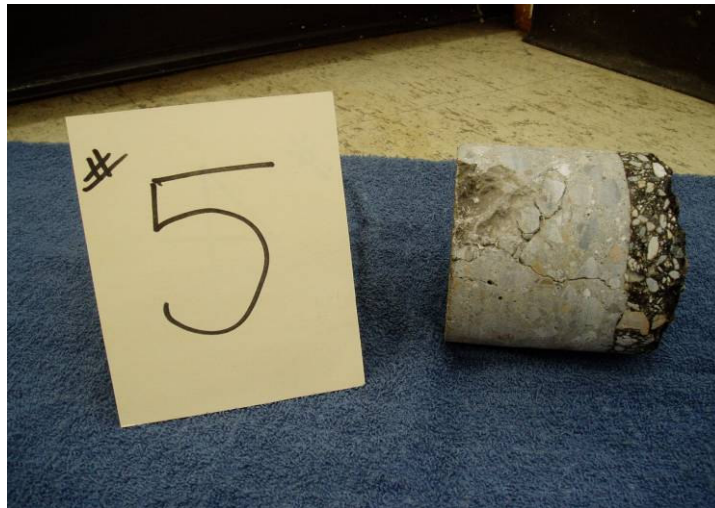
Figure 9. Side view showing cracks and solidly attached HMA. August 2004.
