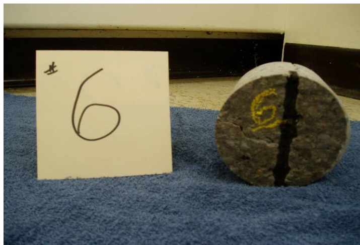
Figure 12. End view showing joint and cracks. 8/04
