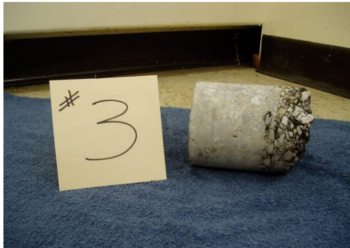
Figure 5. Side view showing whitetopping solidly attached to HMA. August 2004.
