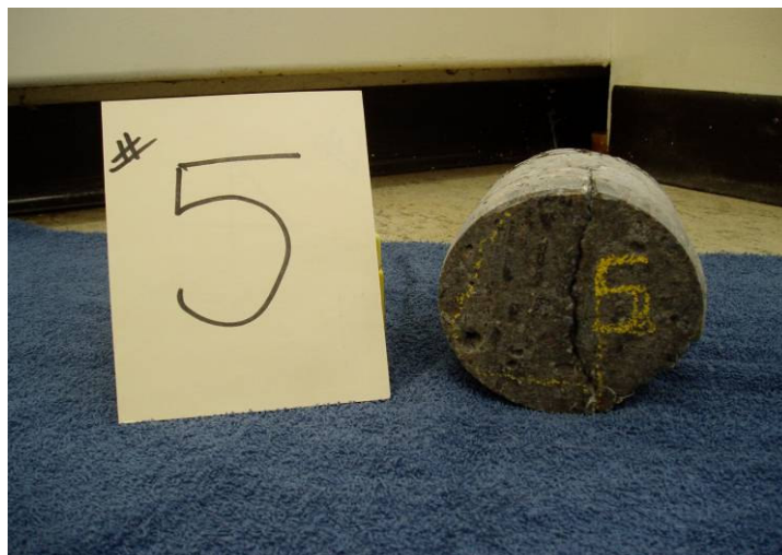
Figure 10. End view showing cracks. August 2004
